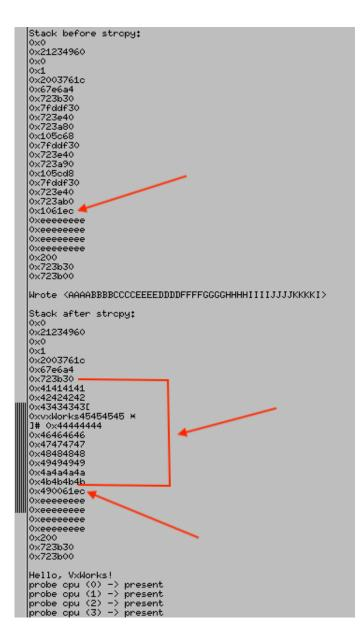
Figure 16: Buffer Overflow Test – 45 character copy
