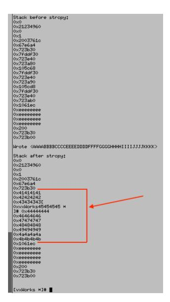
Figure 15: Buffer Overflow Test – 44 character copy
