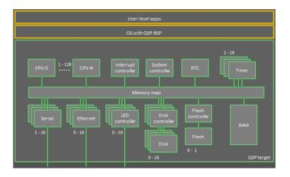
Figure 10: QSP PowerPC Board Architecture
