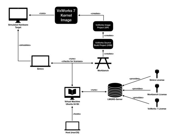
Figure 7: Simulation Setup
