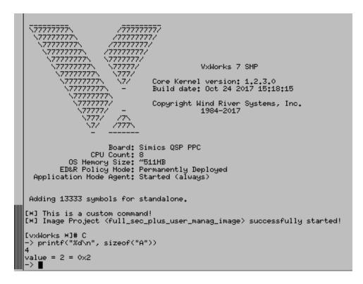
Figure 14: Size of the string "A" on the VxWorks 7 machine
