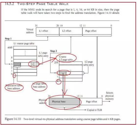
先贴出原代码 (arch/arm/mm/mmu.c), 该函数的功能描述如下: Create the page directory entries and any necessary page tables for the mapping specified by `md'. We are able to cope here with varying sizes and address offsets, and we take full advantage of sections and supersections.
